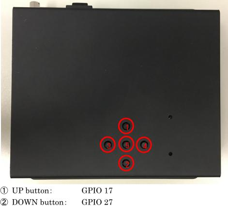
14. GPIO Assignment of General-purpose buttons
