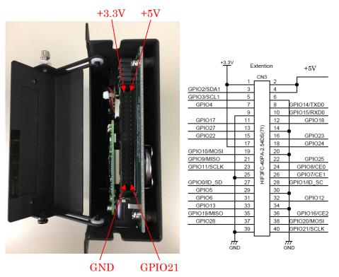
5V of I/O connector turns "ON" when the OS starts. 5V can be turned ON/OFF by the value state of GPIO16.
