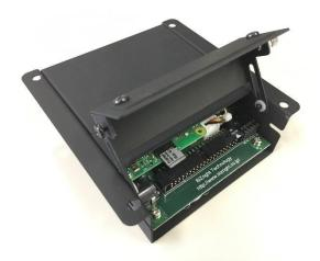
Open the slide lid and insert the Micro SD card directly into the Raspberry Pi.
